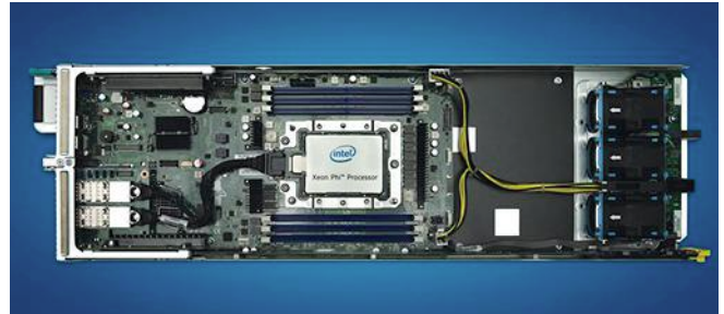
2. Intel’s Xeon Phi is bootable and has Omnipath connectivity support.
