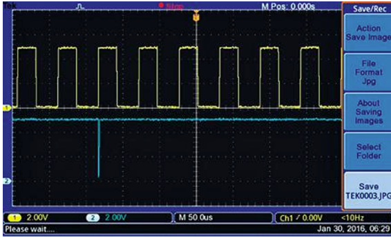
2. A frequency of 18 kHz is received by the down counter (CD40103), and the ZERO pulse is detected when the counter reaches zero.
