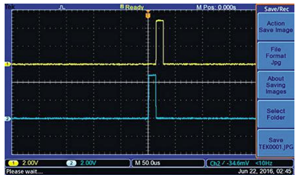
6. These Latch and Reset pulses were generated by the two half-monostables (IC7).
