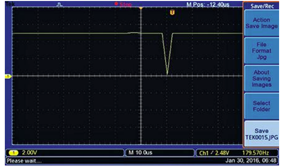
3. The zero-detect pulse indication is provided by the down counter.
