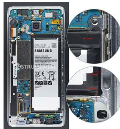
This look inside a Galaxy Note shows the tight XY clearances to the battery. (Courtesy of Instrumental)
